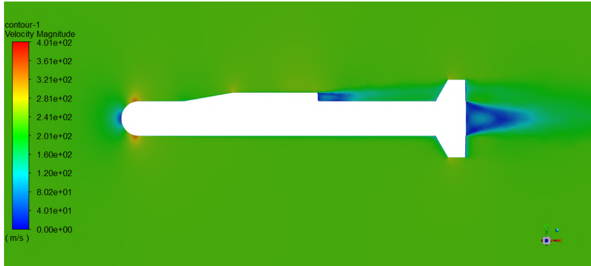
Figure 9: Velocity Contour of Missile at 0^\circ Angle of Attack Before Revision at y/D=0
